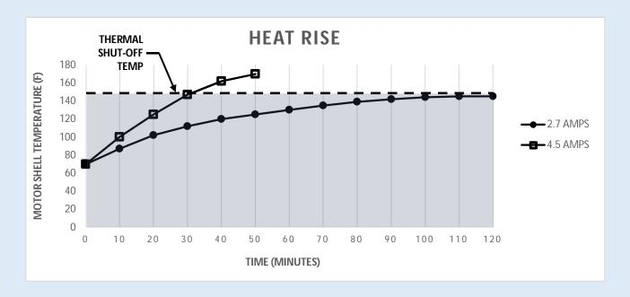
The lower curve of the Heat Rise graph plots the highest current where this pump model can run without a cooling requirement. The upper curve represents the highest current draw of this pump model, under which the thermal breaker would open after approximately thirty (30) minutes and the motor would require approximately twenty-five (25) minutes of cooling before it restarts. Power cycling should be limited to six (6) times per minute.
